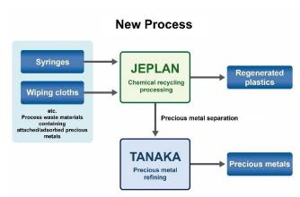
chemical recycling in the future, in addition to the conventional precious metal recovery process through incineration. This initiative is being explored through a business partnership with JEPLAN. The materials targeted for chemical processing include plastics such as syringes and wiping cloths. CO<sub>2</sub> emissions from the targeted precious metal recovery process are expected to be reduced to approximately 10% of conventional levels.
