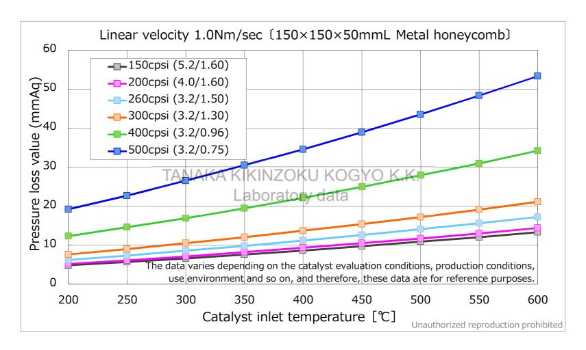
Pressure loss characteristics at various cell densities. For actual design, we calculate the pressure loss value of the actual device based on these characteristics and make a proposal. Please contact us for details.
