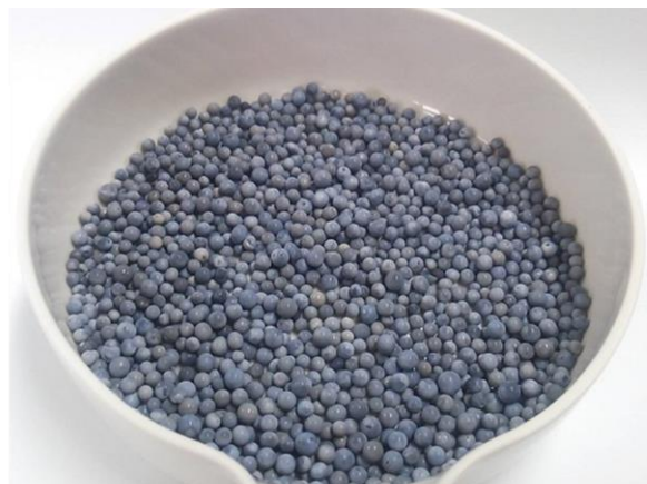
Developed granular hydrophobic platinum catalyst (3mm grain diameter)
