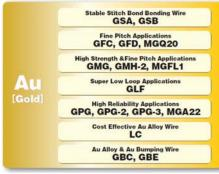
Fig. 1: Typical example of Au wires of Tanaka Denshi Kogyo
