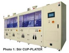
large volume of plating liquid. There are, however, other problems in using these methods. In the case of the first method, for example, it is difficult to attain the agitation effect at the rotation center portion or to protect the cathode contact portion. EEJA's Stir CUP-PLATER has mechanically driven cyclone paddles set in front of the wafer to randomly agitate the plating solution, thereby enabling plating with high film thickness uniformity even at high current densities.
