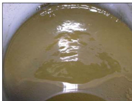
Figure 1: The slurry having sub-micron-sized Au particles being termed "AuRoFUSE".
