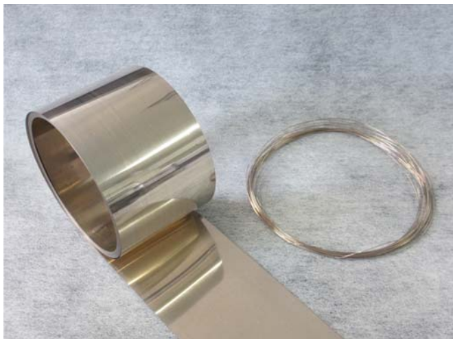
Photo 1: TKC-651 active brazing filler metal
