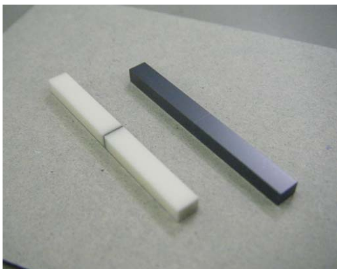
Photo 3: Test pieces for bonding by brazing (Left: Al 2 O 3 , right: Si 3 N 4 )
